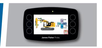
The PME100 range protects operators and assets against overhead structures, including bridges, signs, and power lines. This range of systems provide real time height limitation, using a vertical working envelope, the system monitors the boom and dipper to keep a safe working environment when the limits are set. Hydraulic motion cuts are standard on all PME100 systems to automatically override movement and halt the machine when limits are reached.
