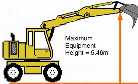
In this example the maximum equipment height is referred to the bucket pin.
