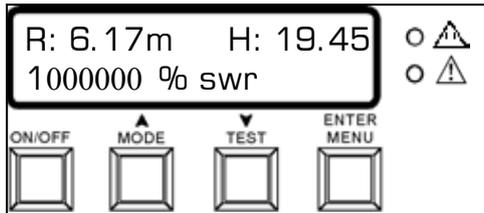
Once the system has completed the initialisation procedure, the safe working radius screen will be displayed.
