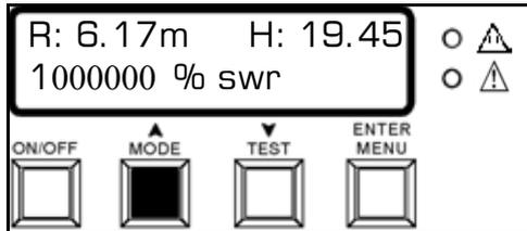
In the safe working radius mode, the tool pivot pin height and radius are displayed. The duty number is displayed in the bottom left corner. The graph represents the distance of the nearest pivot pin to the vertical wall or envelope.
