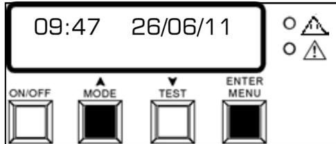
To access the clock setting function, the Rangemaster must be in the Time & Date mode. Press the MODE and ENTER buttons together, the display will now enter the clock set function as described below.
