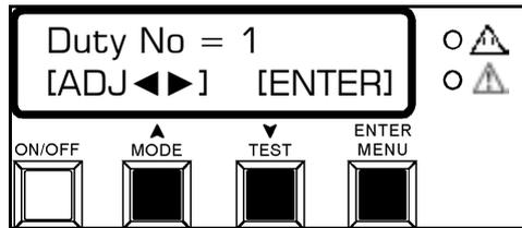
Press ENTER to access the duty change function. Use the MODE and TEST keys to select the required duty number. There is a maximum of 8 possible duty selections. Press ENTER to confirm the selection. After duty changes are made, test equipment to ensure correct operation. The duty number is displayed in the bottom left corner of the SWR screen or use the test function to check current duty and current equipment lengths, see section 6.0.
