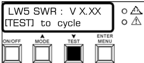
The initial test display is shown here. All information is displayed on the upper line. The lower line contains a scrolling message that says '[TEST] to cycle [MODE] to exit'. This will be present throughout the test procedure.
